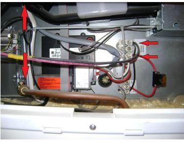
Remove the black and red 10 gauge wires
