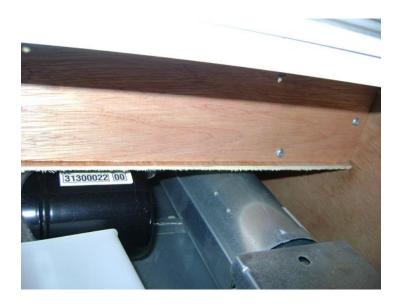
Reconnect 12V and propane line. Test propane line for leak with soapy water.
